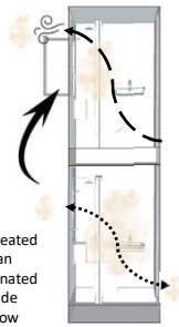
The re-entry of tracer gas due to an open window and the operation of an exhaust fan on the 1/F
